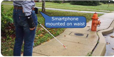
Figure 6: Prototype of the front-end system, RTVision. It is implemented in a generic smartphone and utilizes the camera, the GPS sensor which is used to trigger the camera, and the Wi-Fi module used to download the contextual database.
