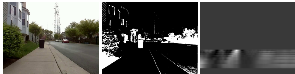
Figure 9: An example of distance-based multi-scale matching. The first one is the image to be searched in. The second image is the segmented image generated by the approach described in the previous section. The last one is the final response of convolving the custom template in the segmented image in distance-based scales. The convolved output provides a likelihood map in which further detection can be operated on high-probability areas only.
