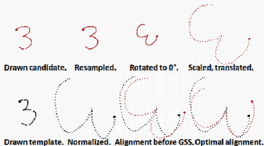
Figure 2. Steps in the $1 matching process and the aligning of a candidate and template. GSS means Golden Section Search .
