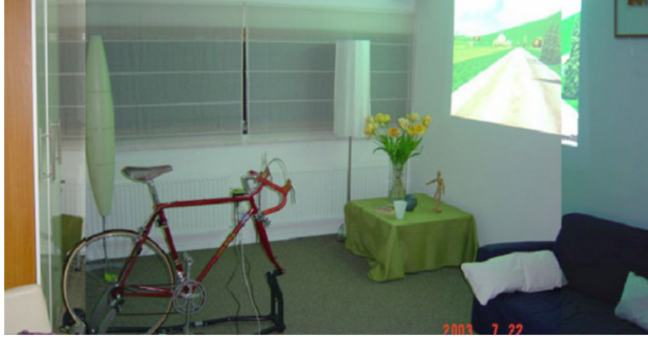
Fig. 1. Composite photograph of the experimental setup, with the stationary racing bicycle placed in front of the wall-projected virtual environment. Participants' viewing distance was approximately 2.20m, with an image size of 1.60m by 1.10m.
