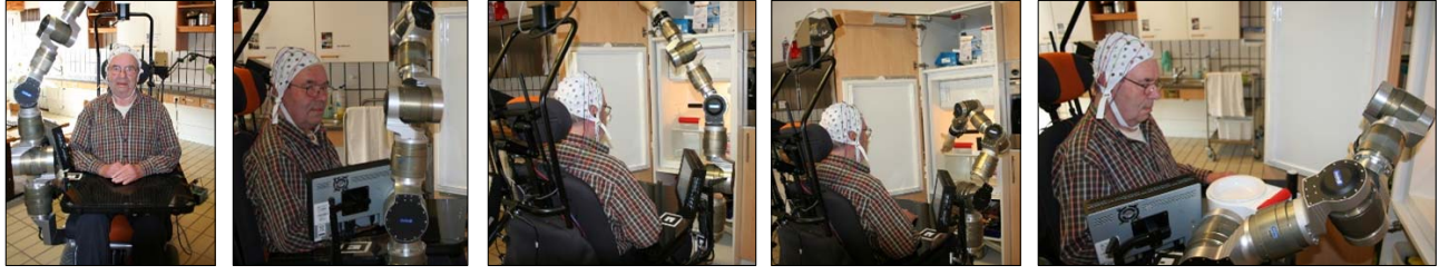
Fig. 11. Sequences of robotic operations within the “prepare and serve a meal” support scenario during testing at the NRZ rehabilitation center.
