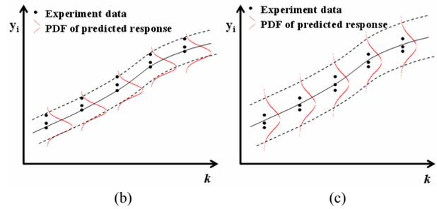
Fig. 2. The concept of the likelihood function in the statistical calibration method (a) High likelihood function; (b) Low likelihood function due to deviated mean values; (c) Low likelihood function due to large standard deviations.
