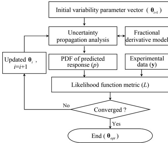
Fig. 3. The procedure of the statistical calibration method.
