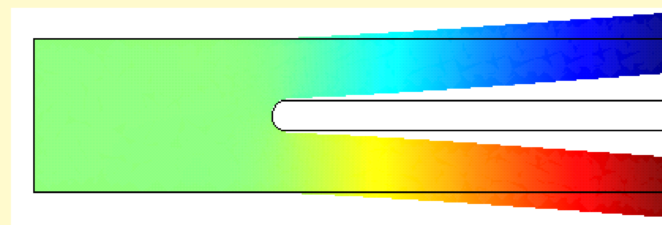
32.8 kHz eigenmode of vibration of QTF
