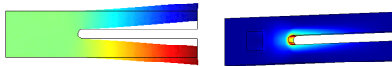
Left: The displacement of the 32.8 kHz tuning fork. The red and blue colors show the maximum and minimum displacement, respectively. Right: The first principal stress. The stress is largest (red) where the tines of the tuning fork meet the base.
