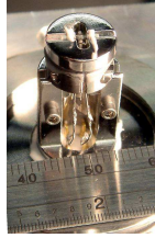
Left: Actual QEPAS sensor device. Right: Schematic diagram of QEPAS device for simulation.
