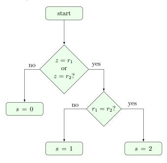
To state the flowchart in words: If z matches neither of  $r_1$  or  $r_2$ , then s = 0. If z matches only one of  $r_1$  or  $r_2$ , then s = 1. If z matches both  $r_1$  and  $r_2$ , then s = 2.
