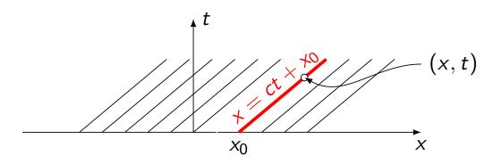
We have seen that the solution w is constant along the characteristics. Thus, referring to the picture above,  $w(x, t) = w(x_0, 0)$ .
