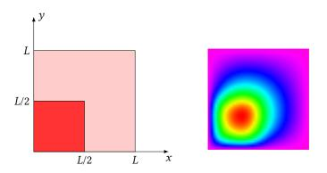
The red square in the diagram on the left shows the part of the plate that is being heated. The picture on the right shows the resulting temperature distribution in the plate according to my calculations. Can you produce a picture like that based on your calculations? That will be get you 5 bonus points.
