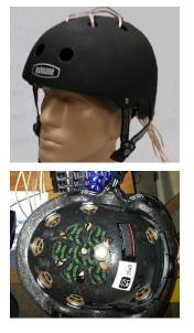
Figure 2. The outside and inside of the current headmounted tactile device prototype [7].
