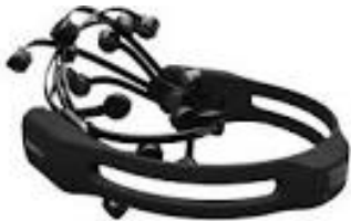
Figure 1. Emotiv EPOC device. Data from 14 EEG channels can be collected to determine emotional information, conscious thought and identify subtle facial gestures made ( www.emotiv.com ).
