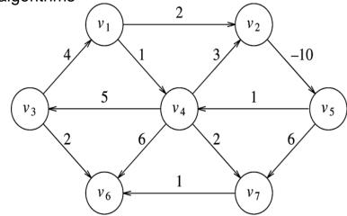
Does not work for above graph, as it has negative-cost cycles
