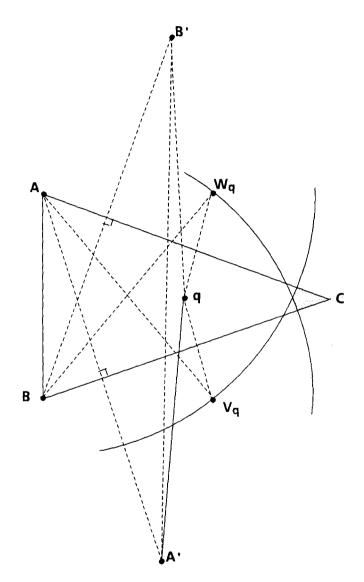
Fig. 6. Covering points near C with a general point q. The ellipse has foci A and B and major axis equal in length to line A'B'.
