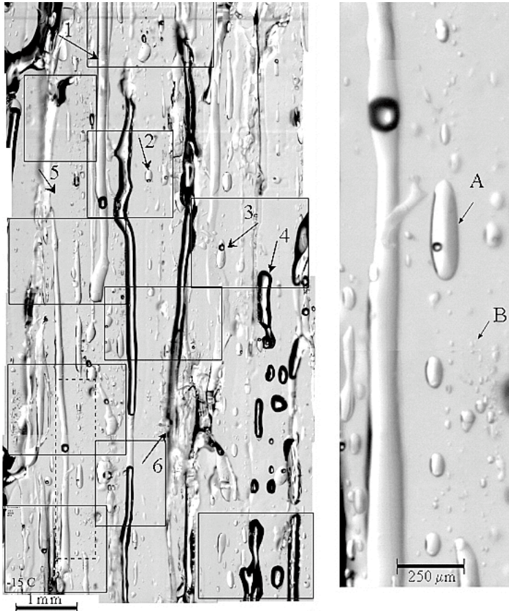
Figure 4. Photomosaic of vertical thin section of first-year ice in transmitted light at -15^{\circ}\text{C} . Ten boxed subregions were used for counting inclusions. Overall dimensions of scene are 12.1 \times 4.7 mm, with 2 mm thickness. Arrows indicate examples of (1) brine tubes, (2) brine pockets, (3) bubbles, (4) drained inclusions, (5) transparent areas, and (6) poorly defined inclusions. (right) An enlargement of box outlined with dashed line. Arrows indicate (A) solitary brine pocket, (B) cluster of small pockets, and (C) string of pockets.
