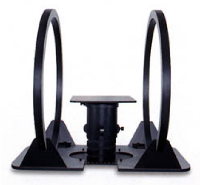
Figure 10: A possible setup of two circular Helmholtz coils. This setup displays two coils with a experiment table in between. A setup like this allows for control of the magnetic field in one direction only.
