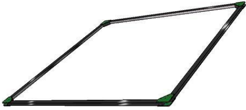
Figure 11: A coil as designed for the Helmholtz cage that is going to be built at the faculty. The coils are squares with sides of about 2 meters. Six coils will be constructed in three pairs. Every next pair will be slightly smaller than the last so the coil pairs can be placed inside each other.
