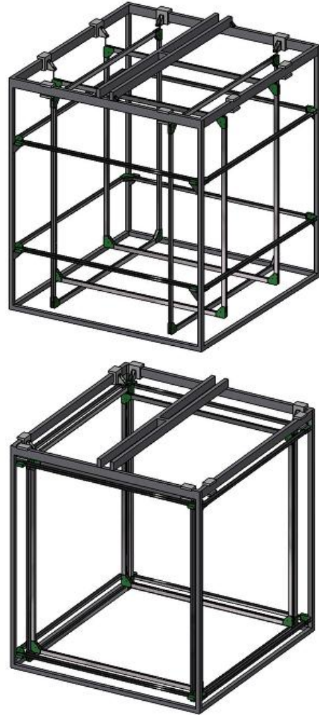
Figure 12: Two possible layouts of the complete Helmholtz cage. The figure displays the design of the complete cage with the support construction surrounding the six coils; one coil pair per axis. On top a layout with inwards shifted coils is displayed. This allows for a test volume of custom size with matching homogeneous field. On the bottom, a layout in which the coils are all shifted to their most outwards position to create the largest possible test volume, but with less homogeneity than with inwards shifted coils.
