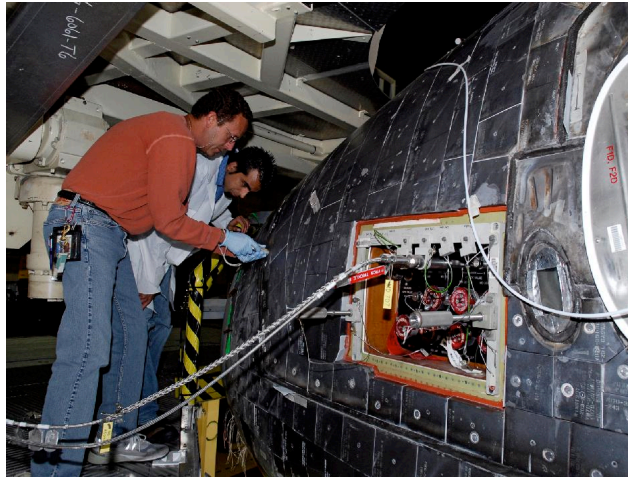
Technicians work on the thermal protection system tiles on Space Shuttle Discovery. On each orbiter are about 24,000 unique tiles, each manufactured with a serial number that identifies that tile's size, shape, and location on the vehicle. Photo credit: NASA/Kim Shiflett
