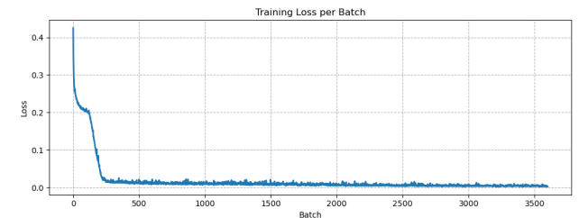
Fig. 12: Training loss curve of U-Net over 120 epochs.
