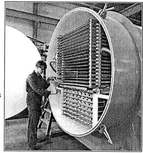
of manufacture and to reduce weight when handling. Each bank is fitted with wheels that run in a stainless steel track located directly above the vapour condenser. Two sets of type 316 stainless steel product trays are provided. These trays feature rounded corners for easy cleaning.
