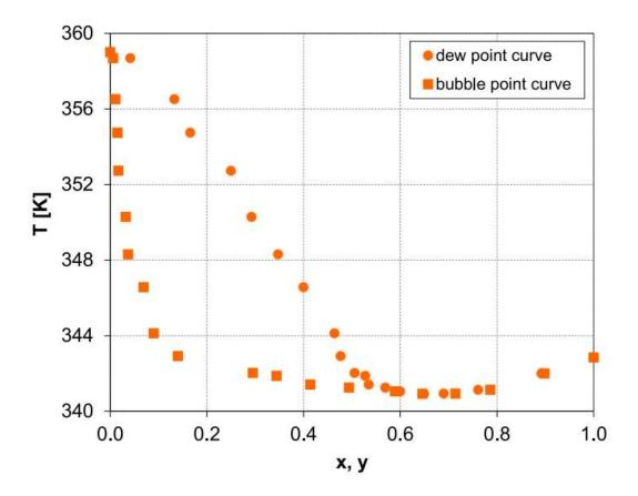
Vapor-liquid equilibrium data for the isopropanol and water binary system at 60 kPa. Note that x and y refer to the mole fractions of isopropanol in the liquid and vapor phases, respectively.
