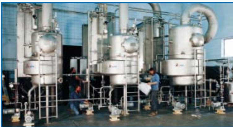
Figure 13. Plant representation. Triple-effect Falling Film Evaporator system followed by a double-effect forced circulation tubular finisher. A distillation essence recovery system was provided to recover the key essence components from the juice and in particular the methyl anthranilate.
