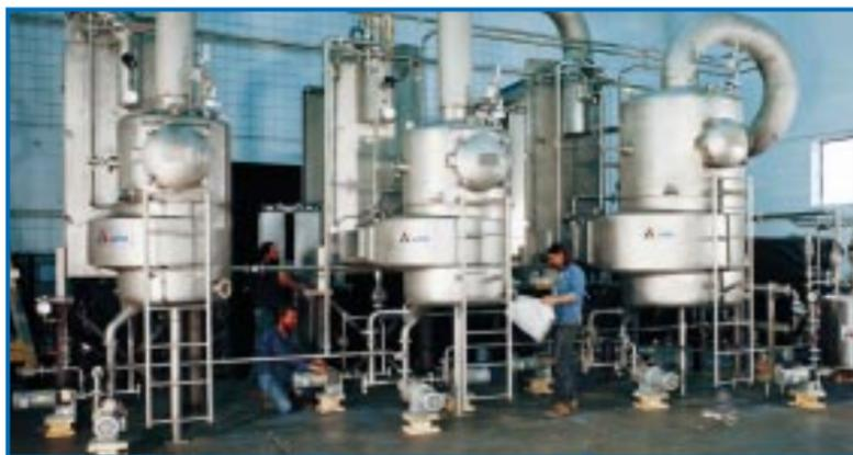
Figure 13. Plant representation. Triple-effect Falling Film Evaporator system followed by a double-effect forced circulation tubular finisher. A distillation essence recovery system was provided to recover the key essence components from the juice and in particular the methyl anthranilate.
