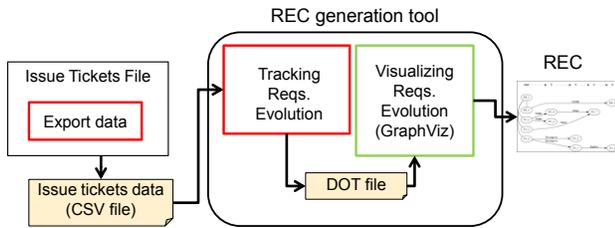
Figure 11. Overview of REC generation tool.
