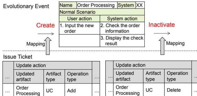
**Figure 4. Create and Inactivate events and the corresponding issue tickets.**
