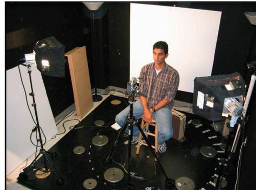
**Fig. 1:** The face image capture setup.
