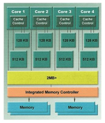
AMD Balanced Smart Cache provides better support for multi-threaded environments with high-speed cache on all four cores.
