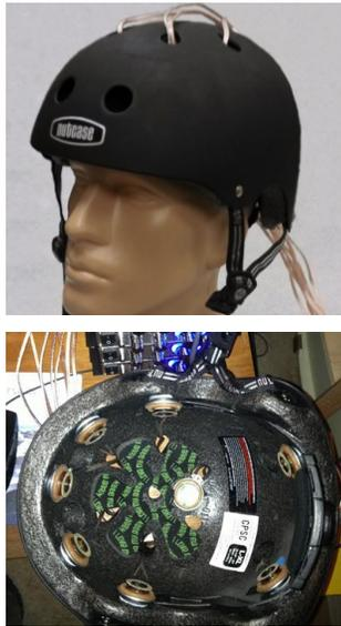
Figure 2. The outside and inside of the current head-mounted tactile device prototype [7].
