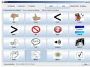
Figure 1: AAC Interface. Each of the 3 screens displays 16 words/icons. Each screen can be accessed via tabs at the top of the interface.
