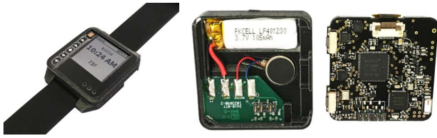
Figure 1: Fully assembled Amulet device (left), Internal Amulet peripherals (middle), custom Amulet circuit board (right)
