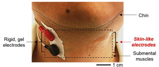
Fig. 1. Imperceptible skin-like electrodes compared to the rigid, gel electrodes: detected surface EMG signals during swallowing are used to drive a biofeedback game.
