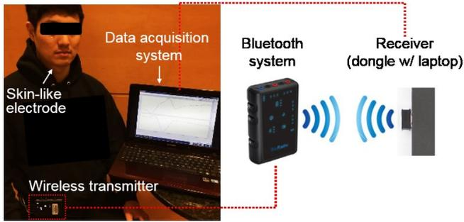
Fig. 3. Skin mounted electrode connected with a standard wireless communication unit for data acquisition.
