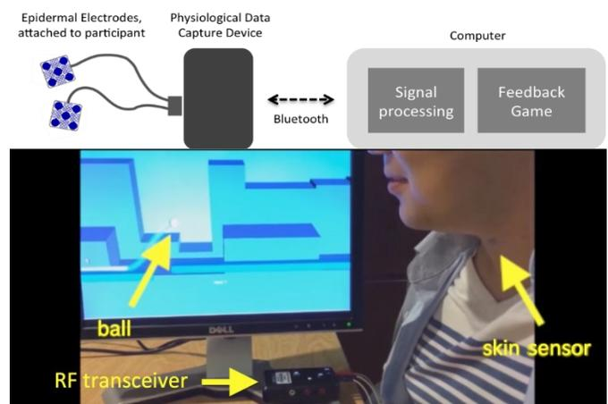
Fig. 2. System architecture showing the skin-like sensors transmitting EMG signals to the computer for a game control.
