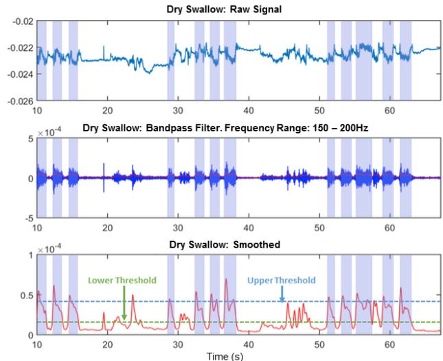
Fig. 4. Representative EMG data (submental muscles) collected using a set of skin-like sensors during swallowing with participant 1: raw EMG signals (top), filtered signals (middle), and smoothed RMS signals (bottom). Shows upper and lower thresholds used to segment the signal and identified swallowing (shaded) segments.
