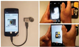
Fig. 2: Prototype of *MT-Diet* application using Nexus 5 and Seek thermal sensor.
