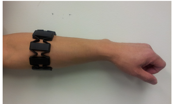
Fig. 1. Myo: An SEMG based gesture recognition device from Thalmic Labs Inc. [3].
