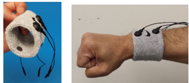
Fig. 2. Our experimental setup: Wrist SEMG band with two signal channels configured using four electrodes.
