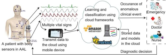
Fig. 1. The scenario of the developed system showing its components.
