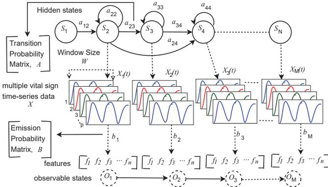
Fig. 4. The structure of Hidden Markov Model and its parameters for multiple vital sign time-series data
