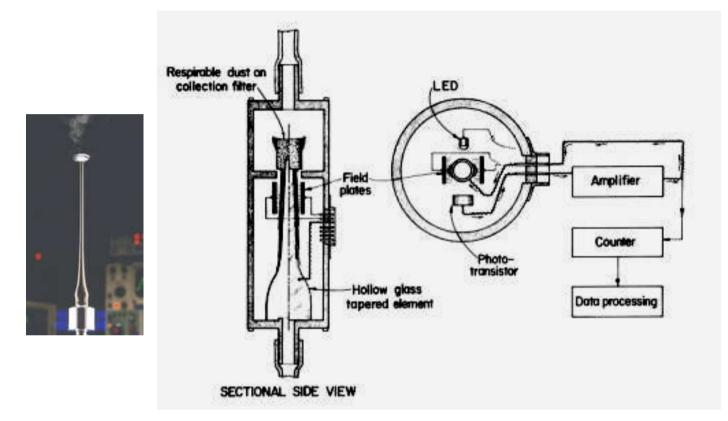
TEOM (Tapered Element Oscillating Microbalance): The particle mass is determined by continuous weighing of particles deposited onto a filter. The filter is attached to a vibrating hollow tapered glass element. The frequency of mechanical oscillation of this element is a function of its mass.
