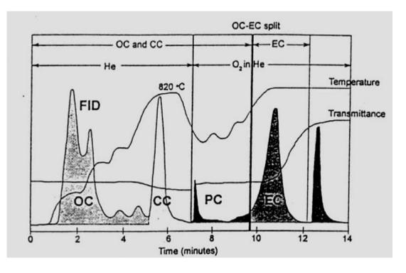
Determination of EC and OC by Thermal Optical Transmission (TOT). The analysis proceeds in two stages:
