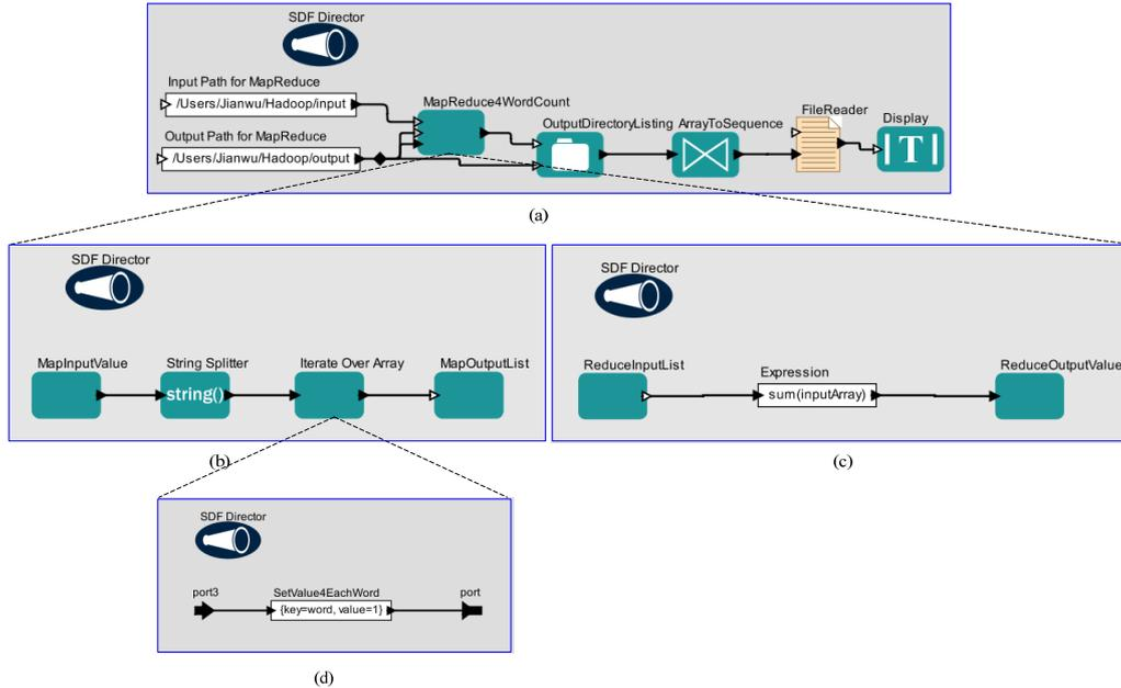
**Figure 4: (a) Word count workflow in Kepler. (b) Map sub-workflow. (c) Reduce sub-workflow. (d) Sub-workflow in the IterateOverArray actor.**
