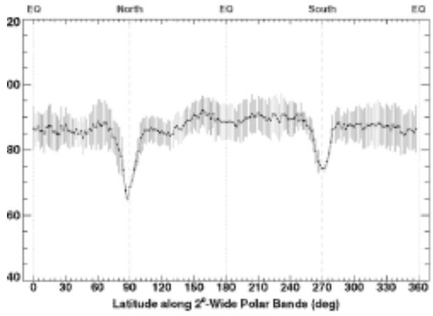
Decreased neutron counts may indicate the presence of hydrogen in water ice
