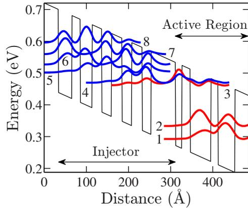
**Figure 2.** Conduction band diagram and moduli-squared wavefunctions of the QCL of [34]. The applied electric field is  $60 \text{ kV cm}^{-1}$ .
