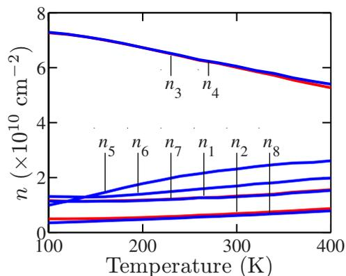
**Figure 4.** Carrier density at different levels versus temperature. The applied electric field is  $60 \text{ kV cm}^{-1}$ , and the total carrier density per period is  $2 \times 10^{11} \text{ cm}^{-2}$ .
