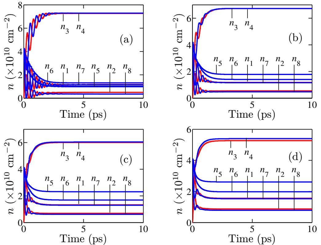
**Figure 3.** Time evolution of carrier density at different levels in the QCL of Sirtori *et al* [34]. The applied electric field is  $60 \text{ kV cm}^{-1}$ , and the total carrier density per period is  $2 \times 10^{11} \text{ cm}^{-2}$ . The temperature is (a)  $T = 100 \text{ K}$ , (b)  $T = 200 \text{ K}$ , (c)  $T = 300 \text{ K}$  and (d)  $T = 400 \text{ K}$ .
