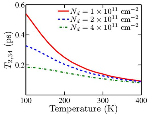
**Figure 5.** Coherence time between the upper lasing level (level 3) and the injector ground level (level 4) versus temperature. The applied electric field is  $60 \text{ kV cm}^{-1}$  and the total carrier density per period is  $2 \times 10^{11} \text{ cm}^{-2}$ .
