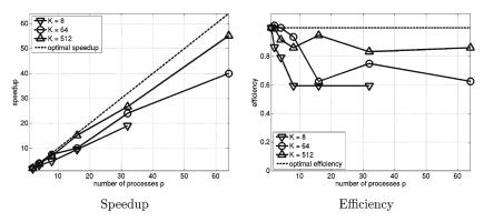
Fig. 8. Speedup and efficiency for 3-D/3-D simulations with  $N_e = 1984$  for Kn =  $\infty$ .
