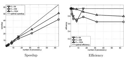
Fig. 7. Speedup and efficiency for 2-D/2-D simulations with  $N_e = 320$  for Kn =  $\infty$ .
