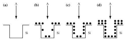
Fig. 2. Schematic of the evolution of deposition of a thin initial layer during chemical vapor deposition.
