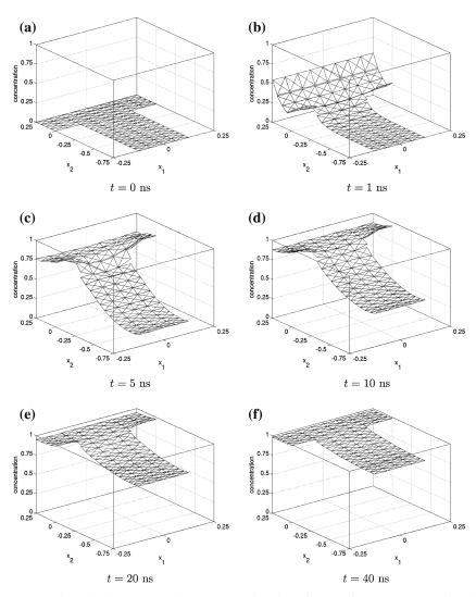
Fig. 3. Dimensionless concentration  $c(\mathbf{x}, t)$  as function of  $\mathbf{x} \in \Omega$  for Kn = 1.0 at selected (re-dimensionalized) times.
