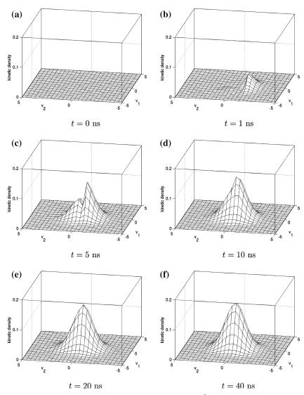
**Fig. 4.** Kinetic density  $f(\mathbf{x}, \mathbf{v}, t)$  as function of  $\mathbf{v} \in \mathbb{R}^2$  for Kn = 1.0 at selected (re-dimensionalized) times. Coordinates of spatial point at the feature mouth:  $\mathbf{x} = (0.0, 0.0)$ .
