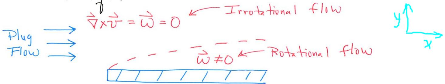
For 2D flow in the  $x-y$  plane,  $\vec{\omega}$  is given as
