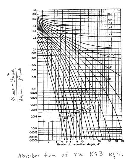
Fig. 2. Absorber form of KSB equation.
