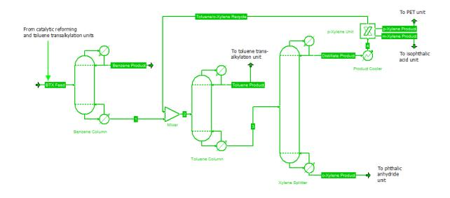
Figure 1. Process flow diagram for BTX distillation sequence (simplified version).
