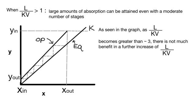
Basic Rule for selecting the flow rate for absorbing liquid:
