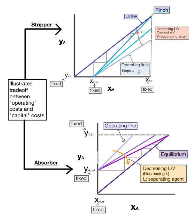
4. Counter current flow is more efficient than co-current flow since in the former, an inlet stream can come to equilibrium with an outlet stream
