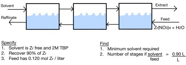
**Example**: Extraction using tributal phosphate in kerosine for recovery of Zr(NO3)4 from aqueous solution
