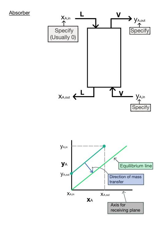
3. Minimum flow of "separating agent" corresponds to an infinite number of plates (staged) or infinite column height (continuous) and to a "pinch" at the feed end.
