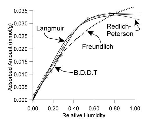
Figure 4. Isotherm Data and Fits for Moisture on Silica Gel.
