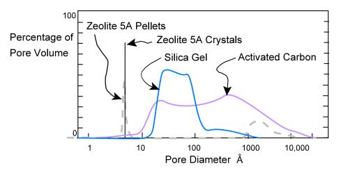
Figure 2. Pore Size Distributions of Common Classes of Adsorbents.
