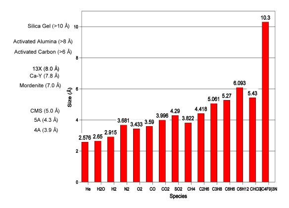
Figure 3. Typical Pore Sizes and Effective Sizes of Common Molecules.
