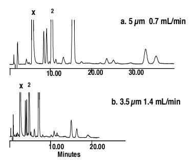
**Figure 1:** Separation of chlordiazepoxide degradation products using a 150 mm x 3.9 mm 5  $\mu$ m Symmetry®  $C_{18}$  column (a) or a 100 mm x 4.6 mm 3.5  $\mu$ m Symmetry®  $C_{18}$  column. The plate count of peak 2 is practically identical for both chromatograms.
