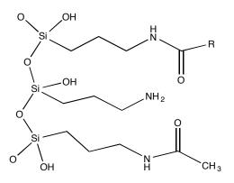
*Figure 2.* Amide phase prepared via a two-step reaction. The phase contains measureable amounts of residual amines.
