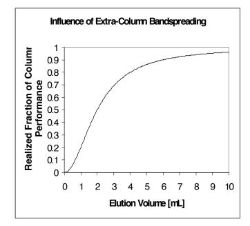
*Figure 1*: *Influence of extra-column bandspreading on column performance*
