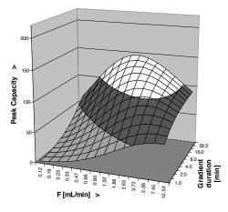
*Figure 1.* Peak capacity as a function of the flow rate and the gradient duration for a  $5 \text{ cm} 5 \mu \text{m}$  column
