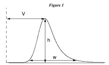
**Figure 1:** Measurement of Extra-Column Volume and Bandspreading. V is the extra-column volume, w is the peak-width at 4.4% of the peak height, corresponding to 5 standard deviations.
